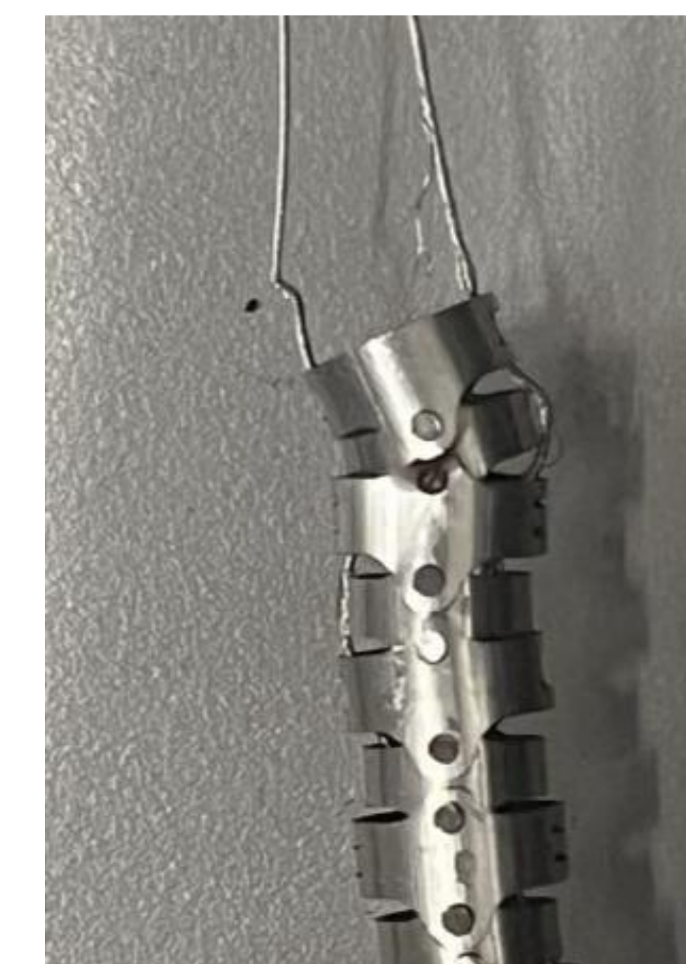
Figure 5: Damage incurred by backbone from compression testing
