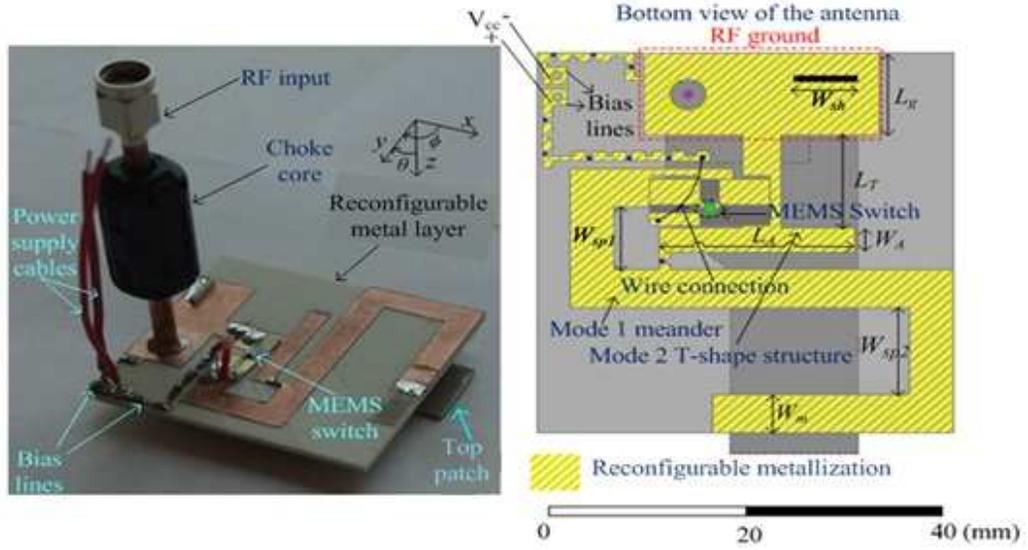
Fig. 3.1: The photographs and schematics of the RF MEMS integrated antenna depicting the critical design parameters.
