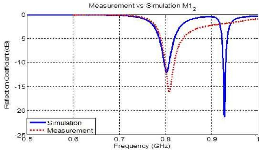
Fig. 4.4: Simulated and measured reflection coefficient plots of the presented antenna in mode 1<sub>2</sub>.
