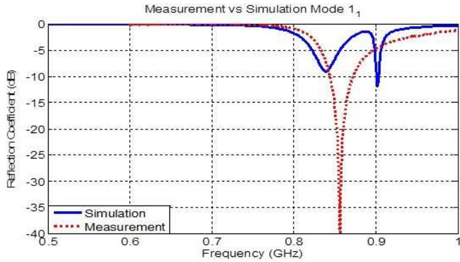
Fig. 4.3: Simulated and measured reflection coefficient plots of the presented antenna in mode 1<sub>1</sub>.
