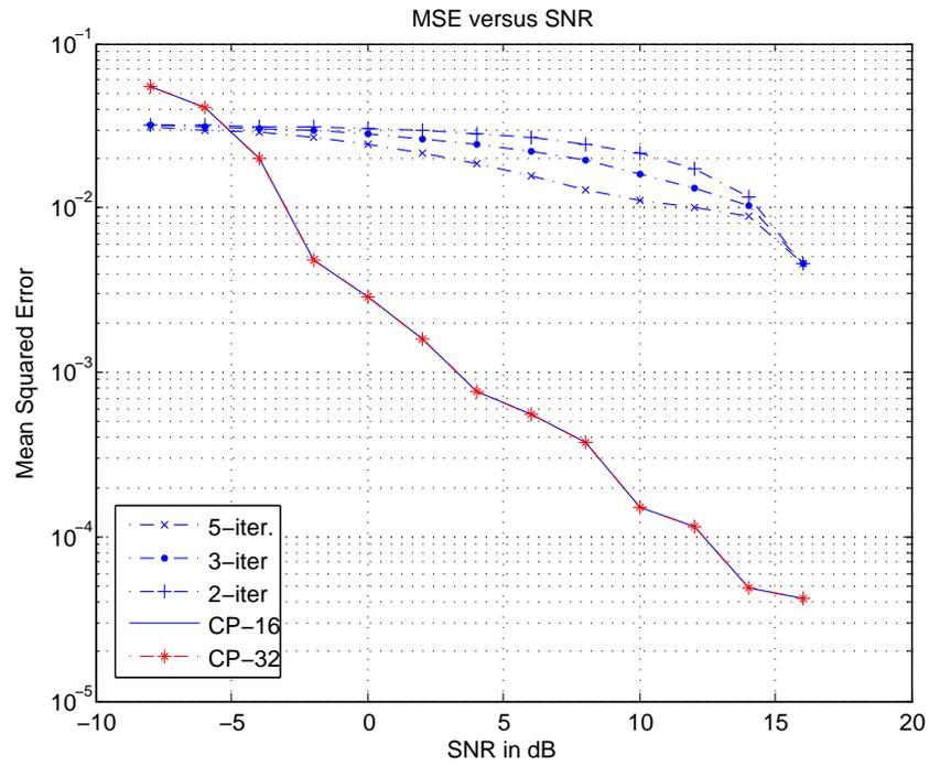
Fig. 3.15: MSE of CFO estimate plotted against SNR.
