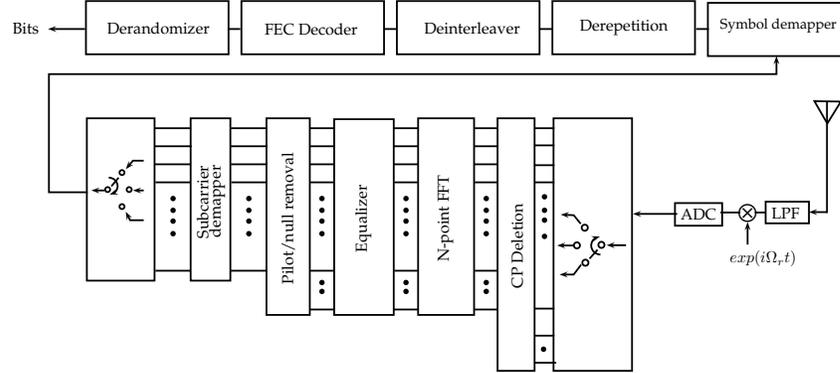
Fig. 1.3: OFDM receiver structure in IEEE 802.16e.
