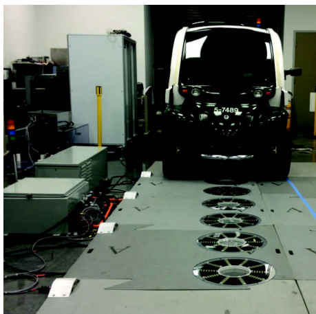
Fig. 1.6: Segmented coils used to demonstrate dynamic charging [8].
