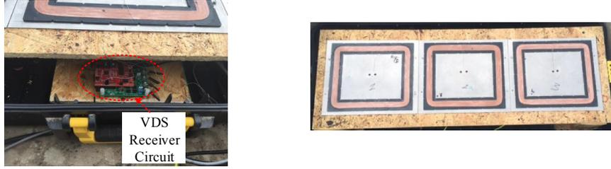
Fig. 3.18: Receiver circuit, and RC structure
