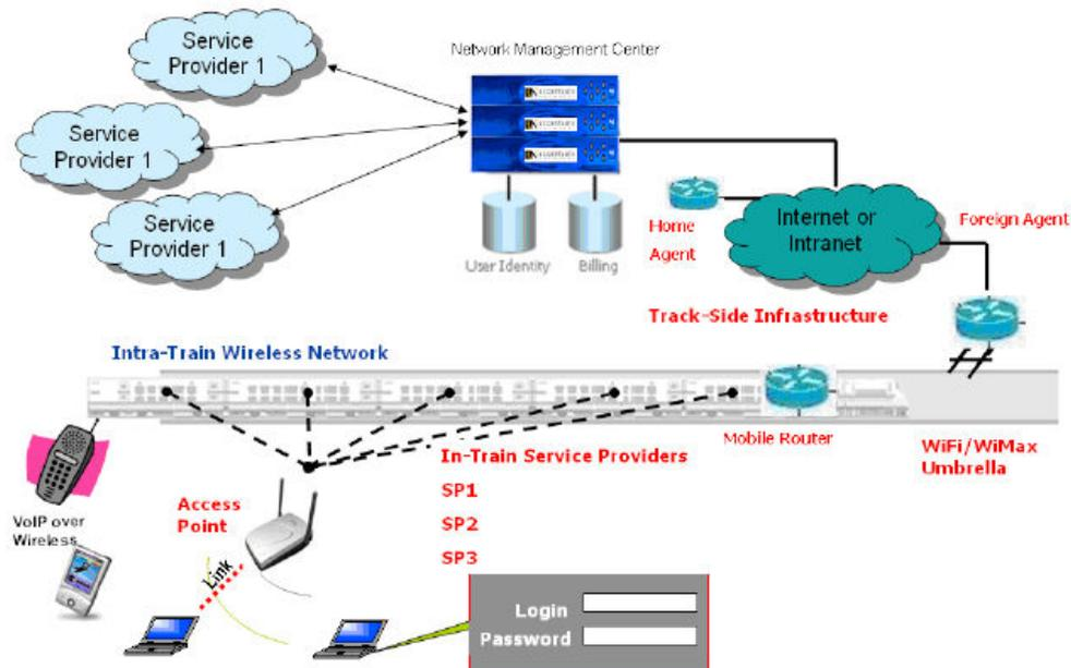
**Figure 3: High Level Network Architecture (Courtesy Cisco Systems).**
