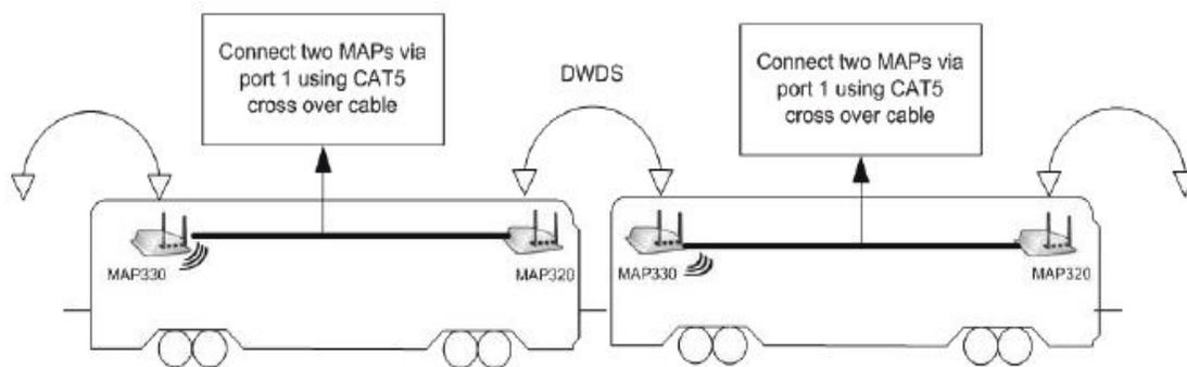
**Figure 6: Inter-Carriage link (Courtesy Colubris Networks).**
