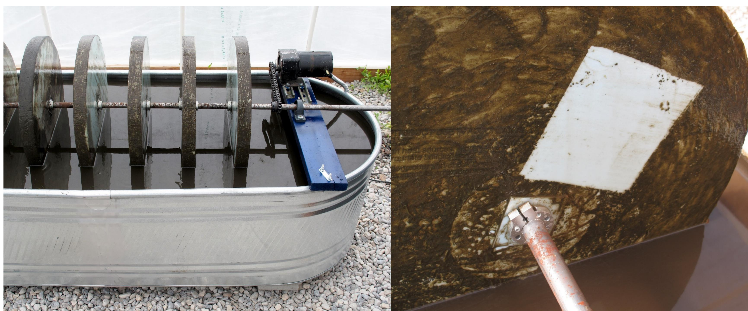
Pilot-scale rotating algal biofilm reactor (RABR)
